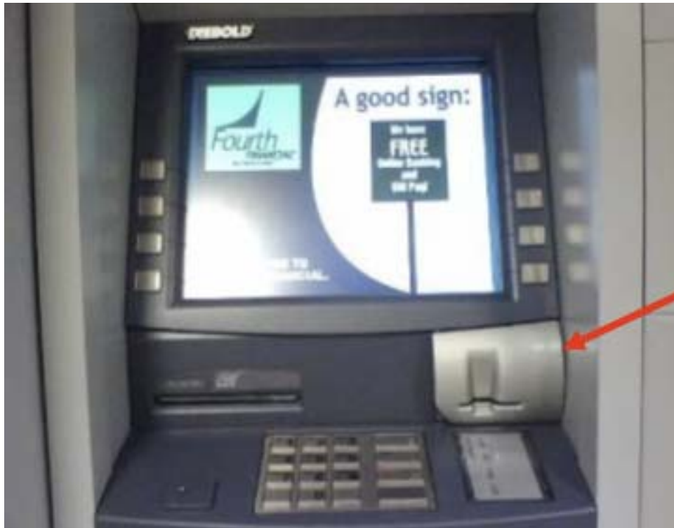
A skim device has been placed on top of the card reader slot. Notice the additional fitted piece that was not in the above photo.
